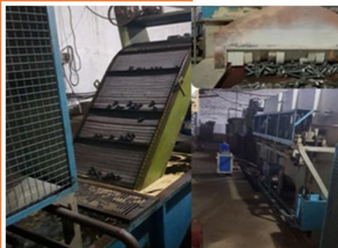
The hardening and tempering process is carried out in fully automatic Continuous heat treatment Plants with logic control. Following Furnaces are installed in our factory.
