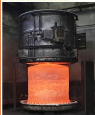
After incoming inspection the raw material is annealed in bell type completely automatic Plc based spherodized-annealing furnace in controlled atmosphere.
